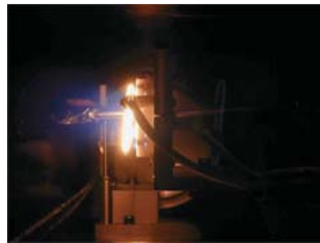
Test firing of a compact plasma accelerator device (Courtesy NASA Glenn Research Center)
